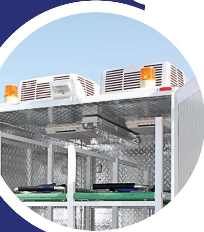
Aerodynamic roof design incorporated with LED warning lights (2 clear flashers & 2 red flashers & 2 oscillators) for greater visibility
